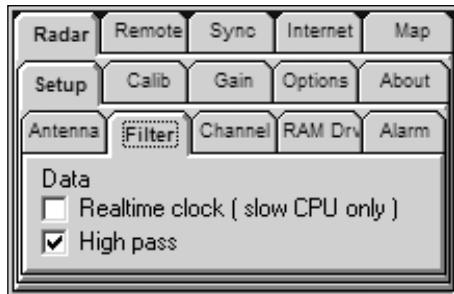
Figure 21 - Selecting a high-pass filter, which helps to eliminate spurious sources
